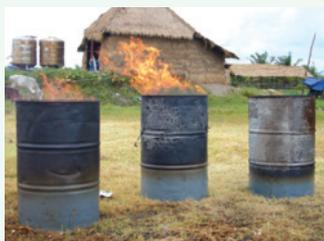
Fig. 21: Acetone burning in 55-gallon drums
