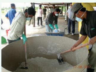
Fig. 17: Preparing the NaHCO<sub>3</sub>/CaO mixture in a tub
