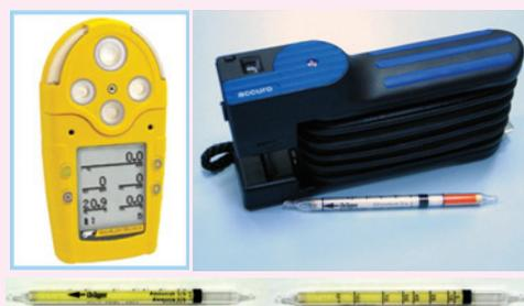
Fig. 2: Combustible Gas Indicator (top left), Drager Pump (top right) and Drager Detection Tubes (bottom right and left)
