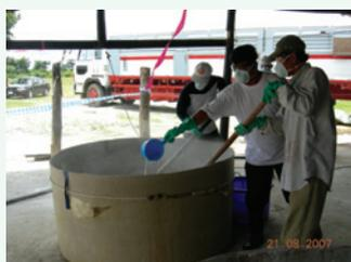
Fig. 18: Pouring the thionyl chloride and hoeing
