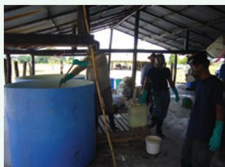
Fig. 22: Neutralization of KOH with conc. HCl
