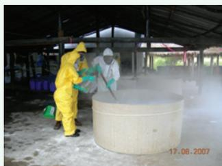
Fig. 20: Adding H<sub>2</sub>O<sub>2</sub> to the neutralized thionyl chloride
