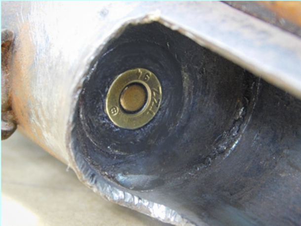
Figure 5: Customized chamber to fit 5.56×45mm cartridge
