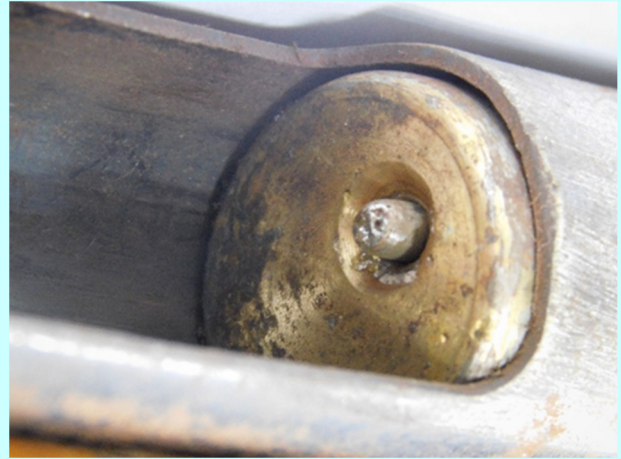
Figure 6: Fabricated firing pin at the air release port
